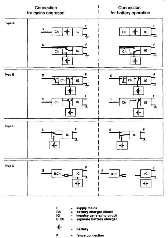
Fig. 101 Schematic Examples of the Different Types of Battery-Operated Energizers Suitable for Connection to the Mains
